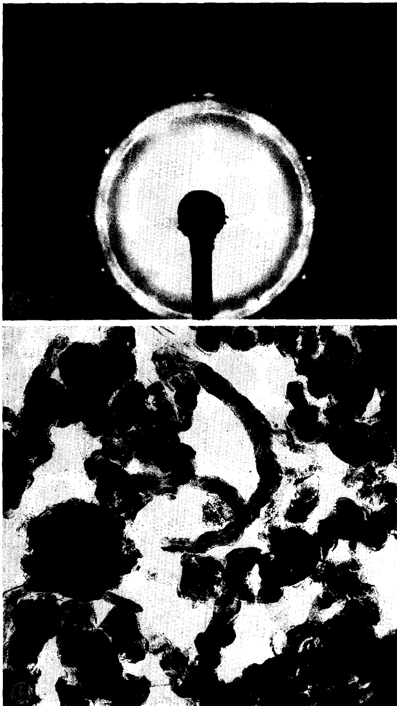
FIG. 11. Selected area diffraction patterns from an area encompassing the growth center shown in Fig. 10. Beam perpendicular to (0001) plane.
