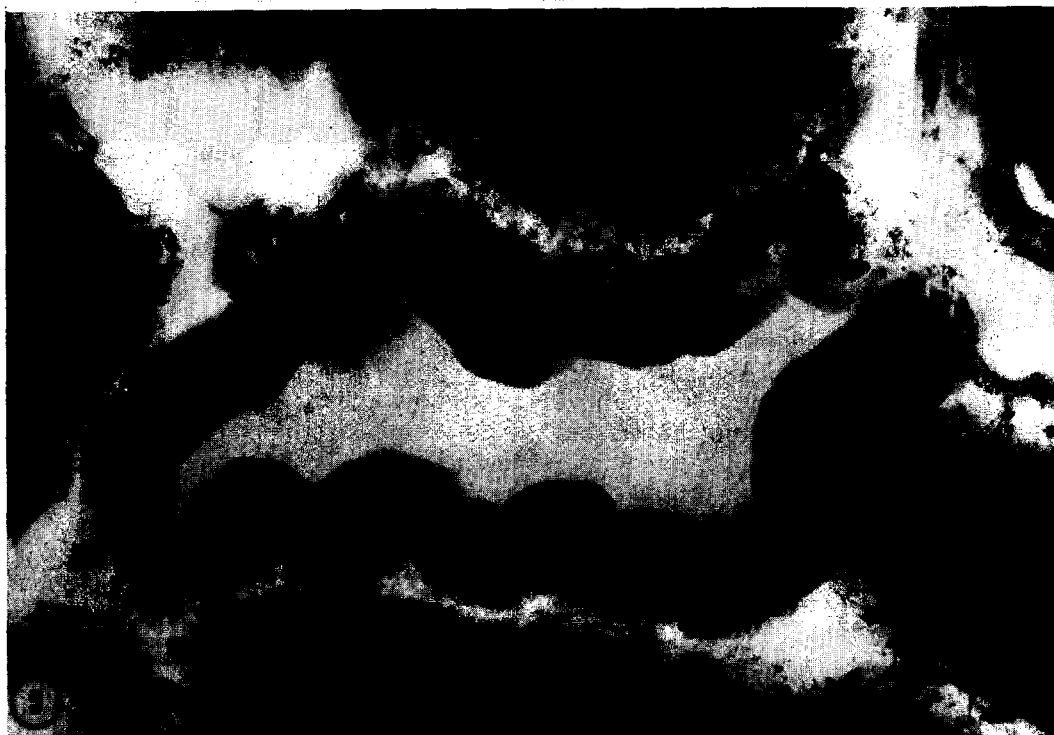
FIG. 4. Transmission electron micrograph showing the film formed on the (111) face of Ni at 800°C in CO-9.4% H 2 . Note the subgrain boundary ABC. (×114 000).
