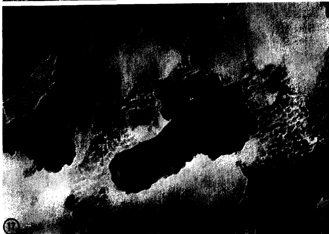
FIG. 16. Transmission electron micrograph of film formed on Co crystal, reacted in CO-9.4% H 2 at 700°C, depicting triangular shaped growth features. (×74 000).
