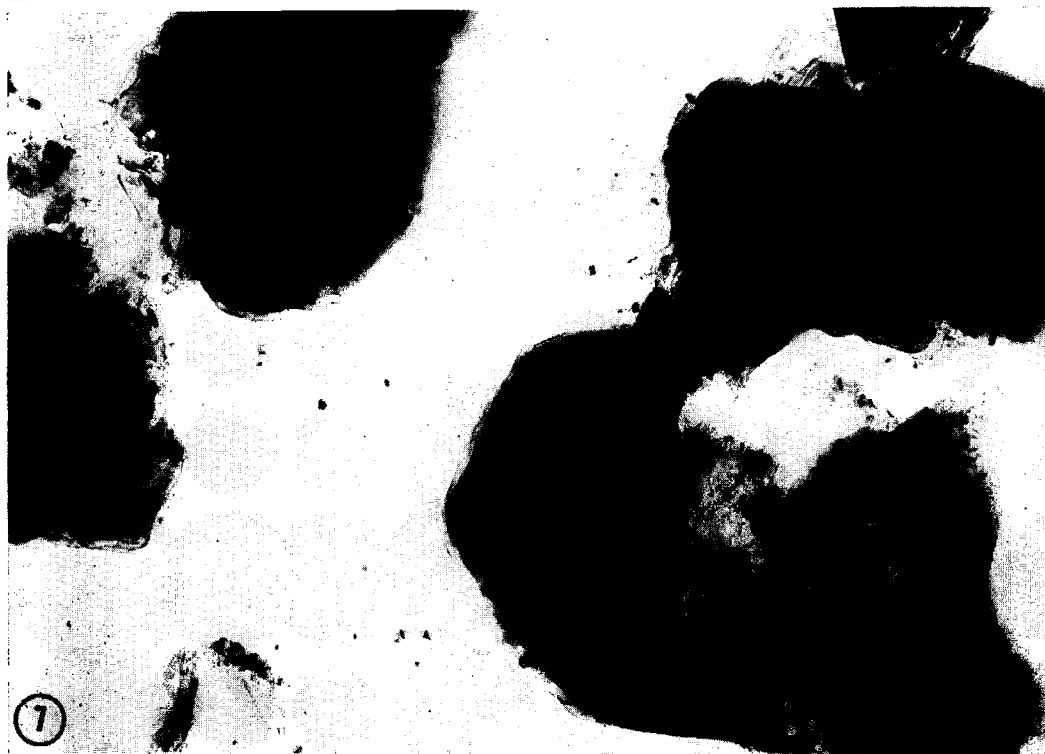
FIG. 6. Moiré patterns and Bragg diffraction contrast effects (see areas A and B) in the film formed on Ni at 800°C in CO-9.4% H 2 . Transmission electron micrograph. ( \times 49\ 000 ).
